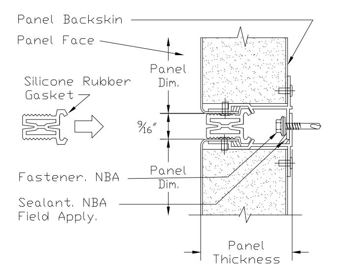
Snug Seam horizontal joint with gasket
